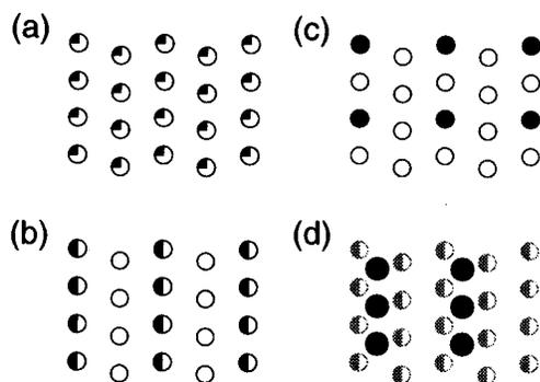
FIG. 5. Schematic of the electronic structures in the surface BEDT-TTF layer: (a) uniform, (b) with twofold periodic modulation along the  $a$  axis, (c) CDW phase, and (d) with a top layer of  $\text{PF}_6$  molecules:  $\bullet$ ,  $\circ$ ,  $\ominus$ , and  $\circ$  indicate 1, 1/2, 1/4, and 0 holes per BEDT-TTF molecule. The large  $\bullet$  in (d) indicate  $\text{PF}_6$  molecules that are completely filled.
