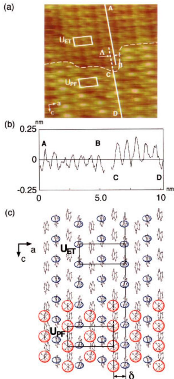
FIG. 3. (a) (Color) STM image of a terrace in Fig. 2(a) ( $10 \times 10$  nm $^2$ ,  $V_s = -44$  mV,  $I_t = 0.53$  nA). (b) Cross sections along A-B and C-D in (a). (c) (Color) Schematic structure of surface shown in (a). BEDT-TTF and PF $_6$  molecules are colored by blue and red, respectively.
