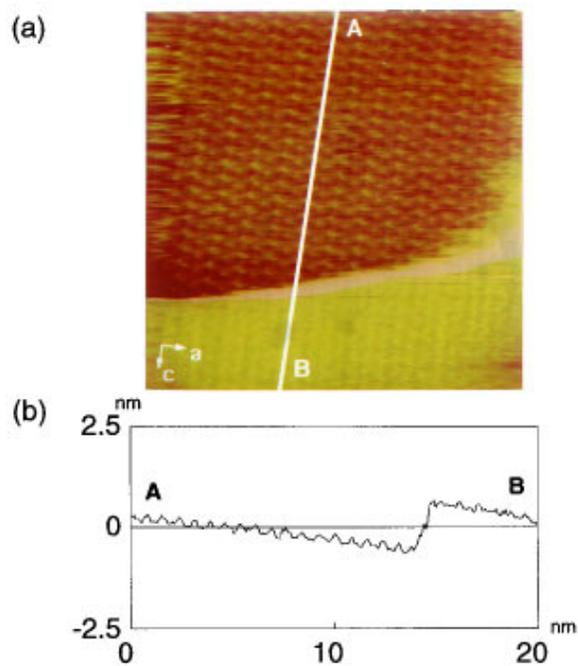
FIG. 2. (a) (Color) STM image of the  $a$ - $c$  plane of  $\beta$ -(BEDT-TTF) $_2$ PF $_6$  ( $20 \times 20$  nm $^2$ ,  $V_s = -100$  mV,  $I_t = 2.1$  nA). (b) Cross section along A-B in (a).
